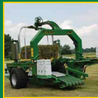
Lifting Bale to Wrapping Position
