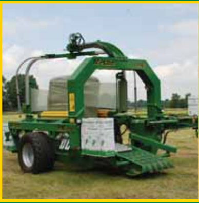
Accurate Rotation of Bale While Wrapping
